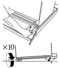
Make sure you lower BOTH REAR ROLLERS. There are two adjusting nuts, one for each roller, at both the front bottom corners of the cooker. Open the grill door and the Tall oven door. Grip under the fascia panel and lift the front of the cooker.
